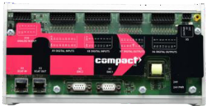
Compact I/O (Guide rail installation)
